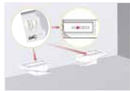
Makes hole from the inside of channel to fix height adjusting sets.
