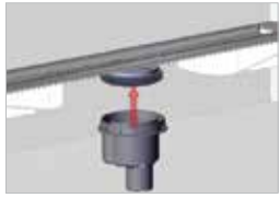
Siphon must be connected to the body.
