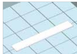
Do not remove the protective styropor until the ceramic application is completed.
