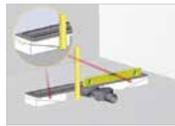
Adjust height adjusting set with scale according to the ground level. Each step is 2 mm.
