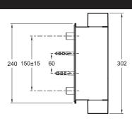
Product Specification: Thermostatic single-lever wall-mount shower mixer. 9104D. Collection: STANCE. Installation: Wall-mount. Connection: With connectors and wall escutcheons. Safety stop at 38°. Maximum temperature 50°. Non-return valves on supplies. Connectors with wall escutcheons.
