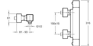
Product Specification: Thermostatic single-lever wall-mount shower mixer. 9096D. Collection: STRAYT. Installation: Wall-mount. Connection: With connectors and wall escutcheons. Safety stop at 37°. Non-return valves on supplies. Connectors with wall escutcheons.
