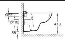
Product Specification: Wall-hung WC pan 54 x 36 cm. 19916D. Collection: ODELA. Dimensions: 54 x 36. Weight: 15.3 kg. Material: Ceramic. Installation: Wall-hung. Projection 54 cm.
