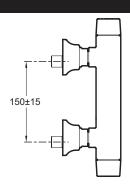
Product Specification: 2-handle wall-mount shower mixer. 16297D-9. Collection: MARGAUX. Weight: 3.4 kg. Installation: Wall-mount. Flow rate: 20 l/min. Hole configuration:  $150 \pm 15 \text{ mm}$ . Margaux offers a unique blend of traditional design elements and modern fluidity to complement eclectic design interiors with refreshed sophistication.
